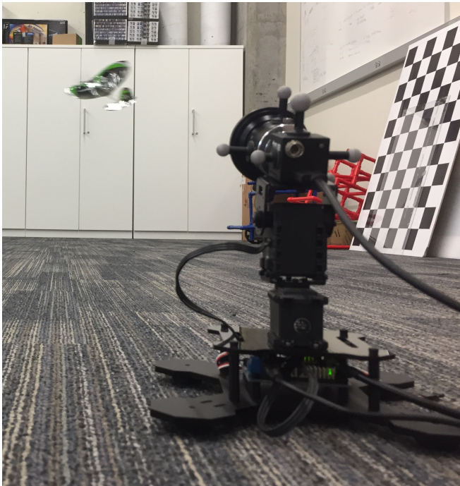
Fig. 4: The result from tracking the Vapor Lite in the motion capture room. Notice that the turret has motion capture dots as well as the Vapor Lite. Their respective orientations are known from the motion capture data and the needed desired pan and tilt for the turret is calculated.
