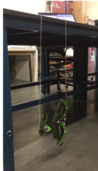
Fig. 3: Photo of capturing the mass moment of inertia. The aircraft is suspended from the table and then swung around its center to get a final inertia result.
