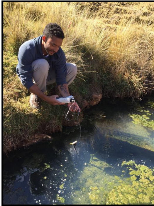
Figure 3. Field measurement of temperature, pH, and conductivity using an Oakton portable meter at Baños Conococha.
