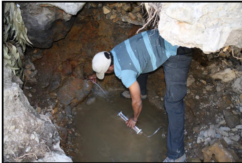
Figure 4. Collection of water sample using Cu tubing equipped with refrigeration clamps at Baños Chavin.
