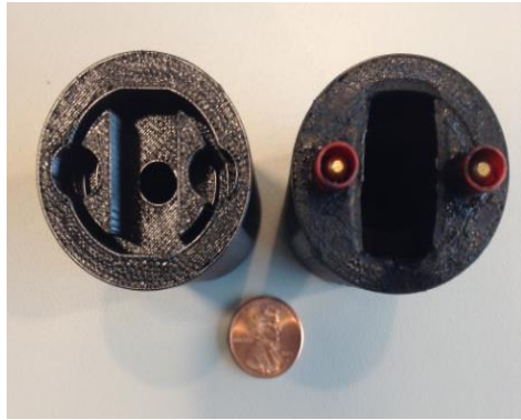
a) Printed Fuel Grain with Electrodes
