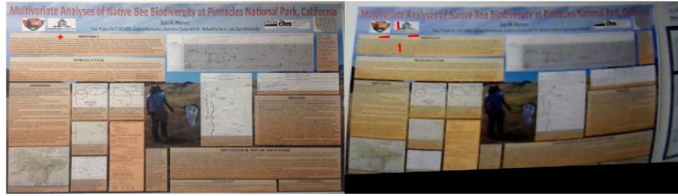
Fig. 2.5: Image registration: the clear photograph of the poster with the calculated coordinate of the crosshair (left) and the transformed poster from the video frame (right)
