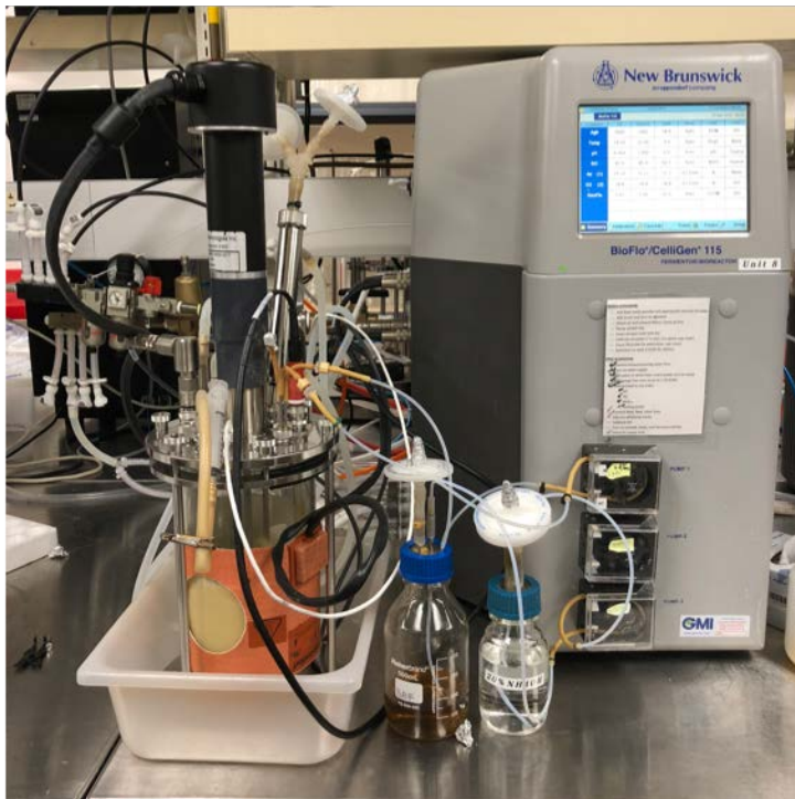
Figure 2-3. Benchtop bioreactor setup for MiSp expression
