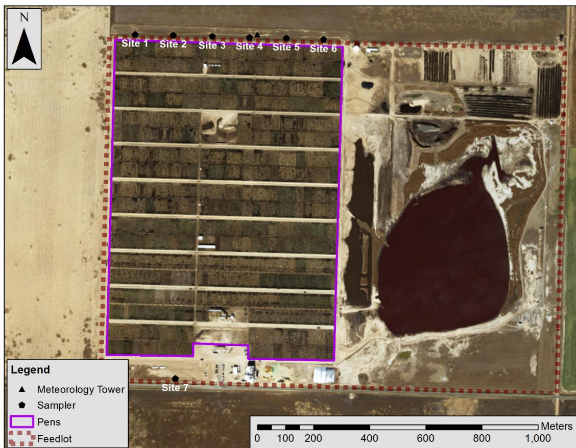
Figure 6-1. Satellite image of the feedlot under study with particle and meteorological measurement locations shown, as well as the facility and pen borders.
