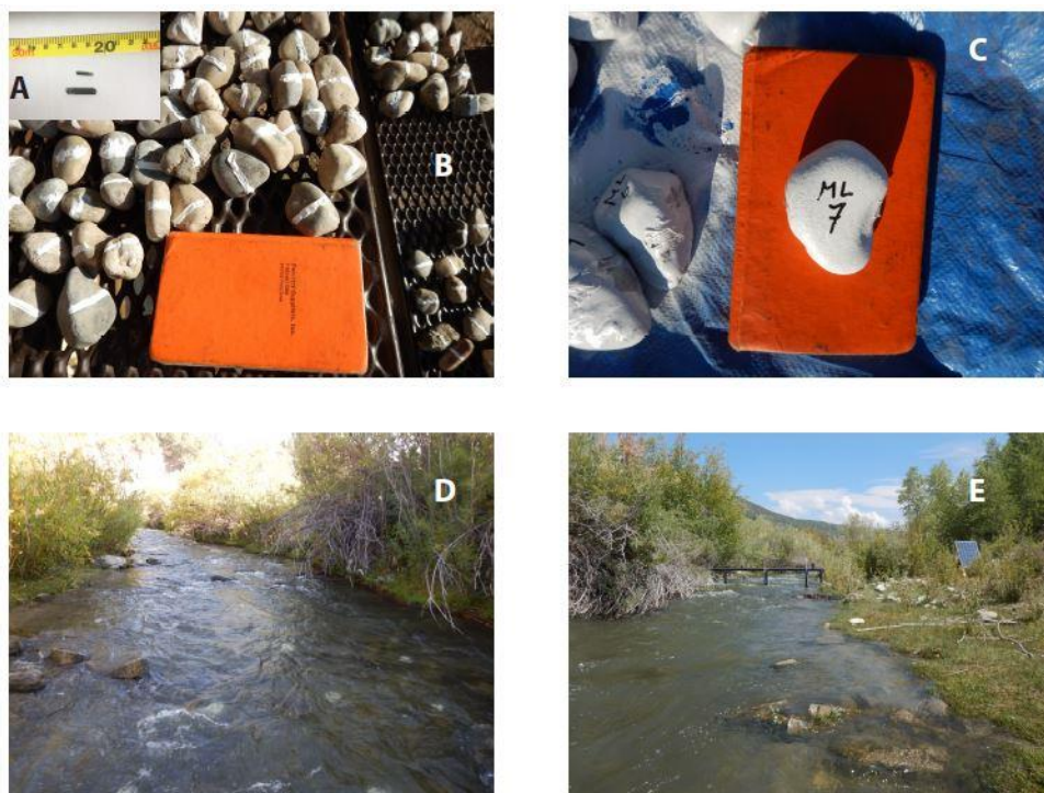
Fig. 3.4. Pictures of the RFID deployment system. A) 23 and 32 mm PIT tags, B) tracers sealed with marine epoxy, C) tracers painted white and labeled to aid in visual detection, D) tracers deployed in the stream, E) channel spanning RFID antenna powered by a solar panel.
