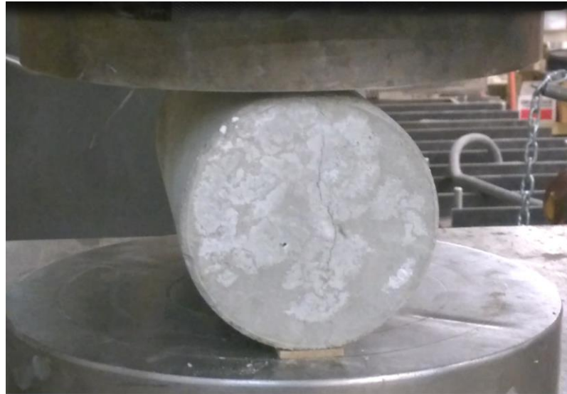
Figure 11 Splitting tensile test
