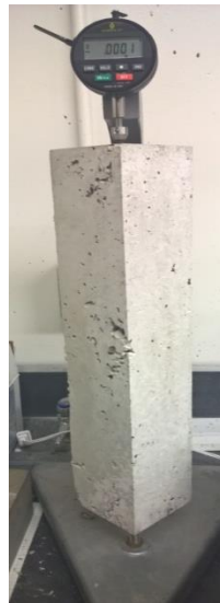
Figure 12 Length comparator for Drying Shrinkage
