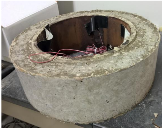
Figure 14 Restrained shrinkage ring test
