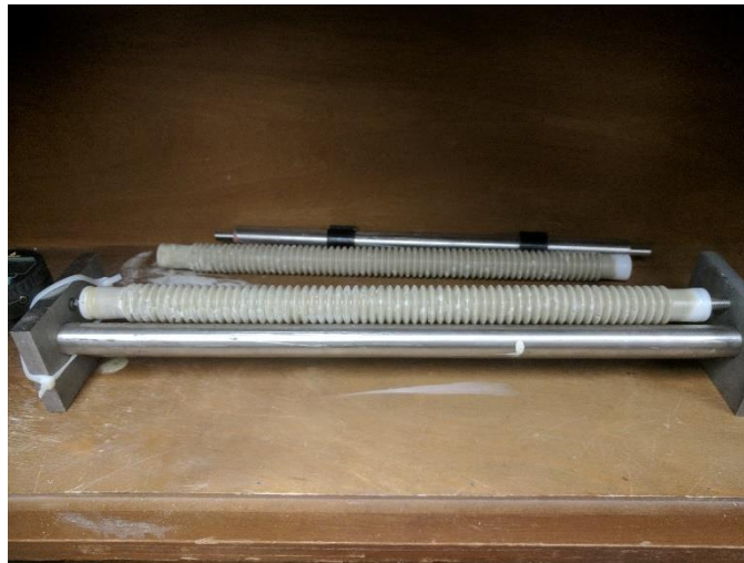
Figure 18 Autogenous shrinkage apparatus
