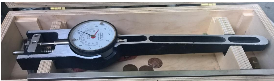
Figure 17 Creep strain gauge
