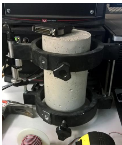
Figure 10 Compressometer for determination of modulus of elasticity
