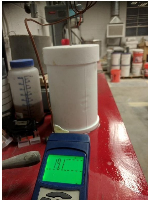
Figure 19 Thermal history setup
