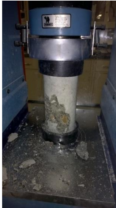
Figure 9 Cylinder in the compressive strength test with neoprene caps
