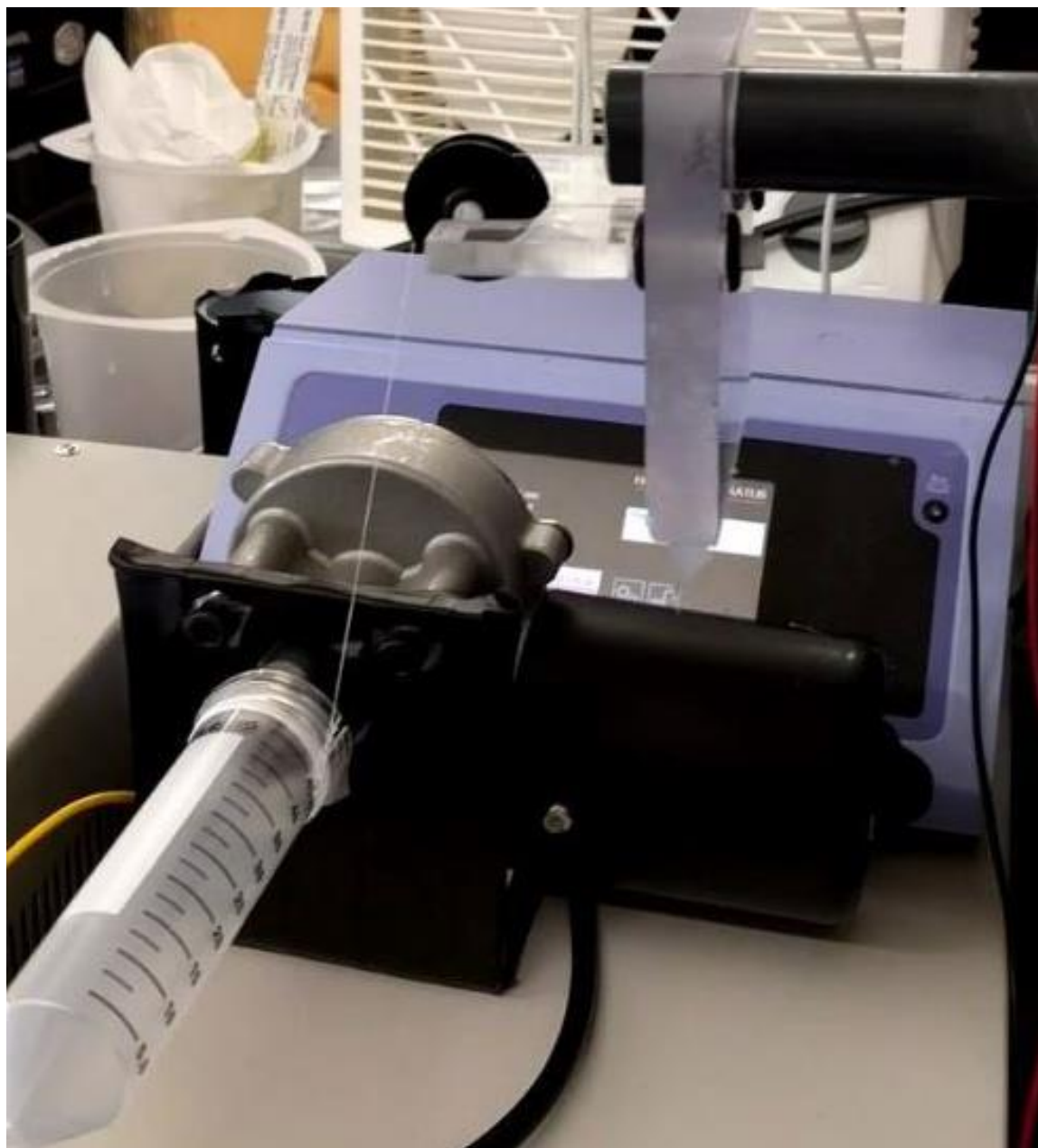
Figure A3: Reeling system for continuous electrospinning
