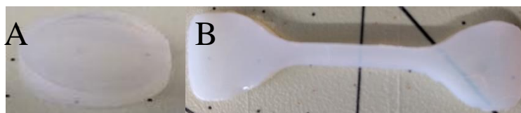
Figure 3.3. (A) Compressed post-treated cross-linked cylindrical hydrogel with no stress fractures. (B) Post-treated cross-linked hydrogel as dog bone for uniaxial tension testing.
