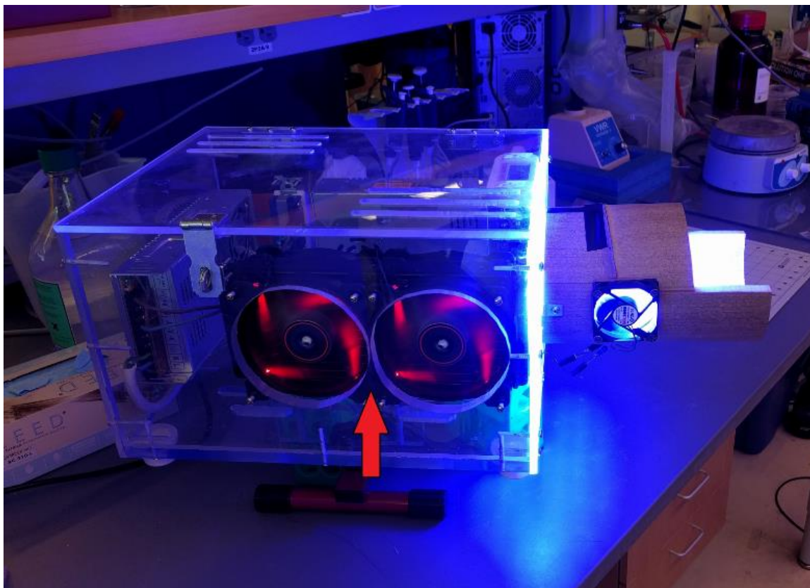
Figure D1: CLIP with 465 nm LED. Red arrow indicates cooling system.
