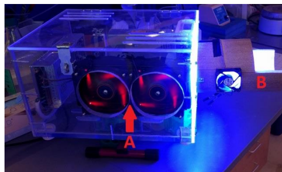
Figure 3.1. CLIP activated. (A) Cooling unit (B) Staging area for samples.
