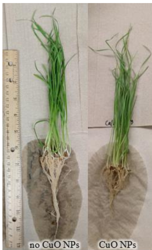
Figure 2-40: Reduction of root length in wheat by exposure to CuO NPs in sand.
