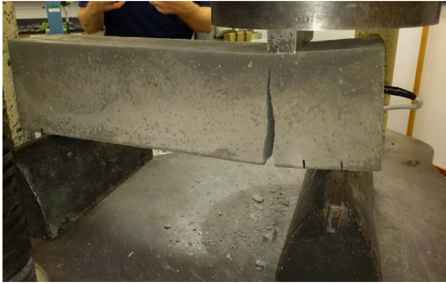
Figure 3-9 Concrete sample after failure
