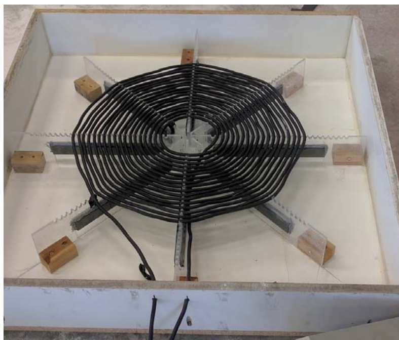
Figure 3-19 Test 5 heat-shrink coated Litz wire
