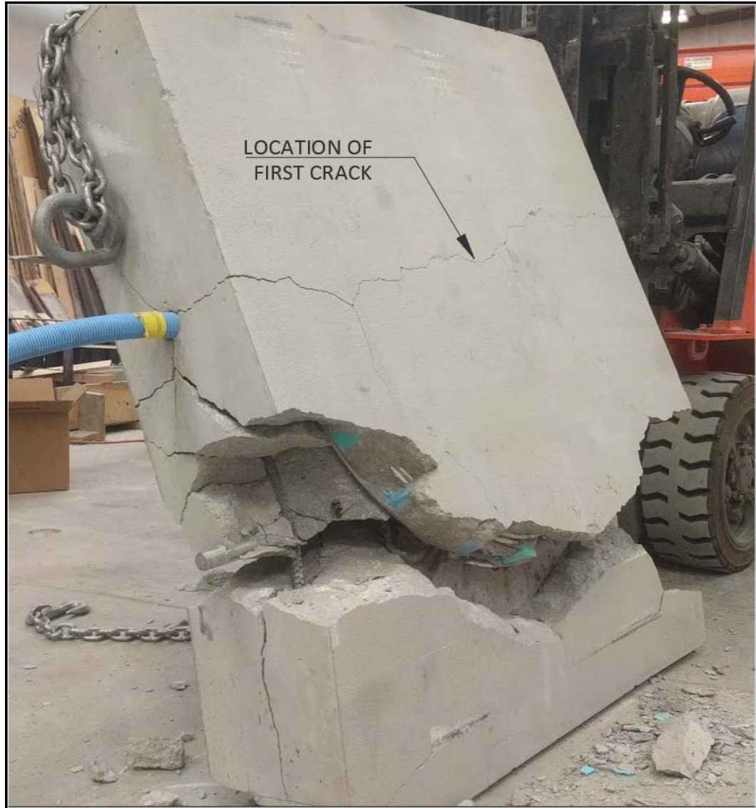
Figure 5-27 Third pad post failure
