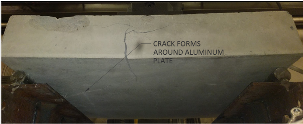
Figure 5-15 Crack 3/8 inch wide, (35,000 cycles)
