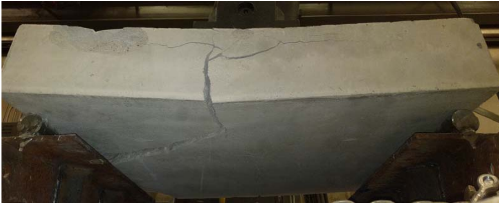
Figure 5-16 Crack \frac{3}{4} inch wide, (36,000 cycles)
