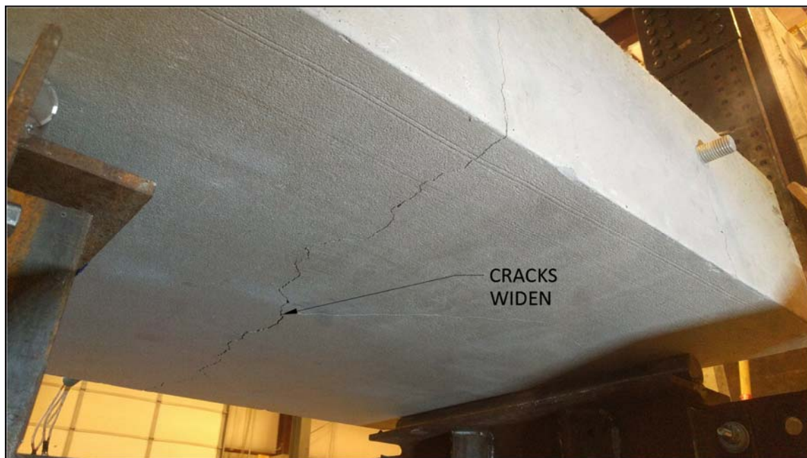
Figure 5-23 Crack 1/8 inch wide
