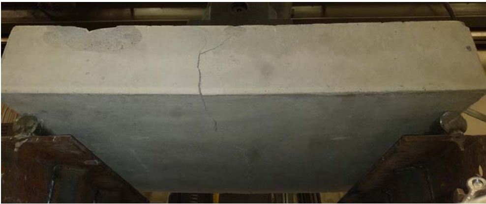
Figure 5-14 Crack 1/4 inch wide, load increased (32,000 cycles)
