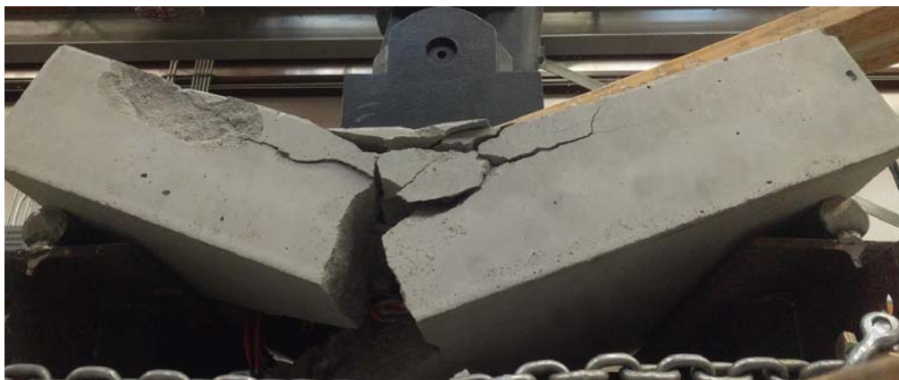
Figure 5-17 Failure (approximately 40,000 cycles)
