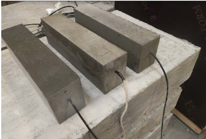
Figure 3-7 Embedded Litz wire segments
