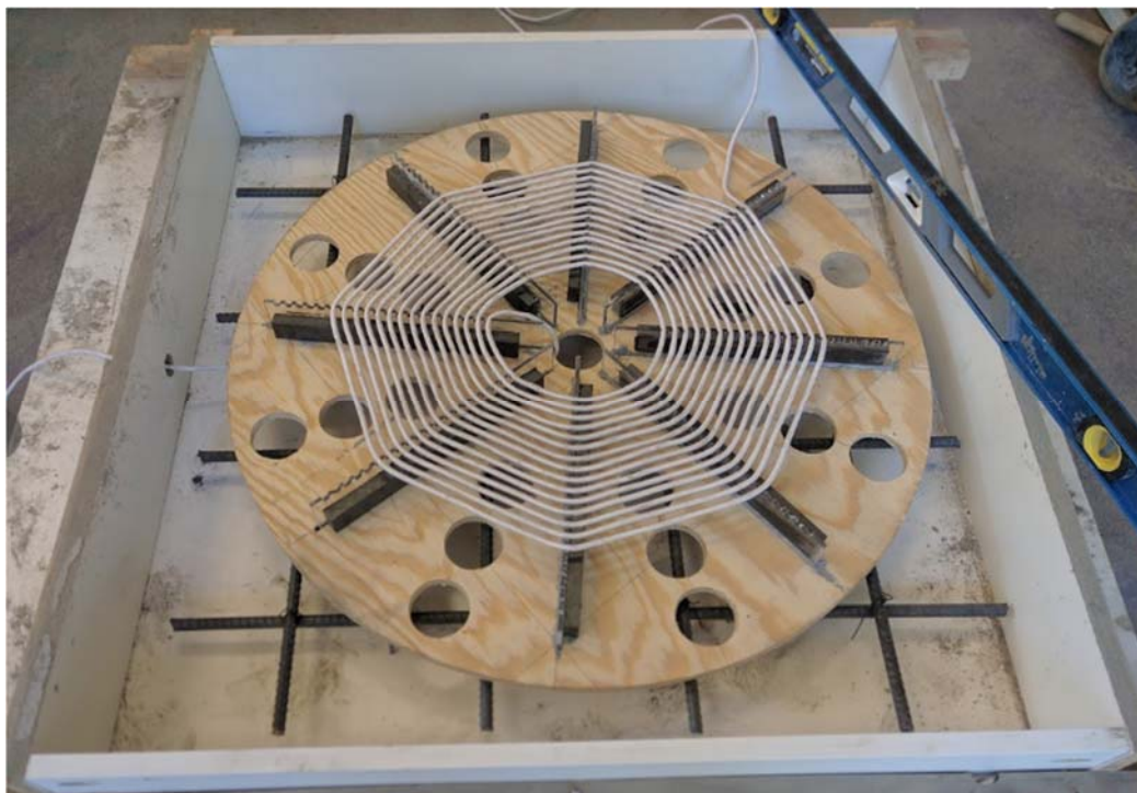
Figure 3-17 Test 3 IPT coil without aluminum plate
