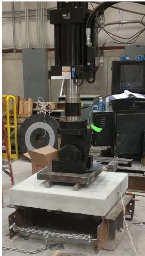
Figure 4-5 Four-point bending test set up
