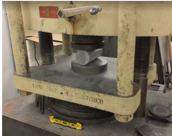
Figure 4-7 Split tension test set up
