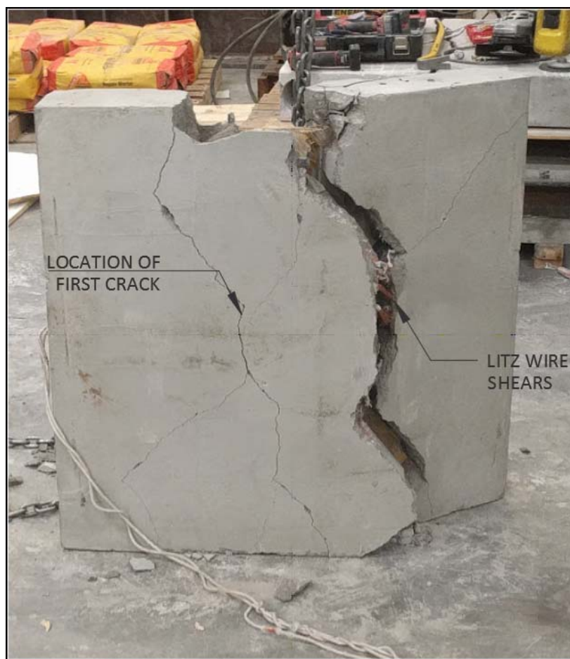
Figure 5-9 First pad post failure
