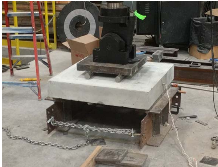
Figure 5-1 First fatigue test set-up
