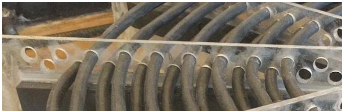
Figure 3-21 Close up of final pad vertically offset wire spacing
