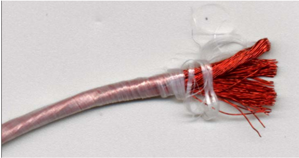
Figure 3-15 Litz wire with nylon sheathing
