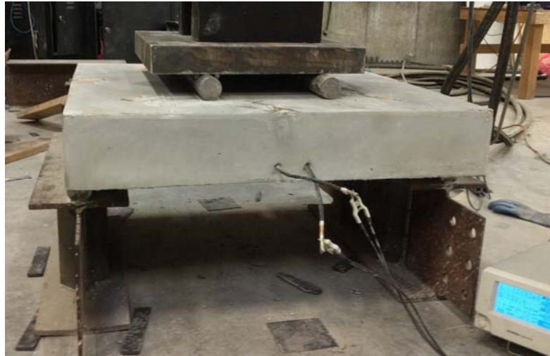
Figure 5-28 Other Sample tested with four-point bending test
