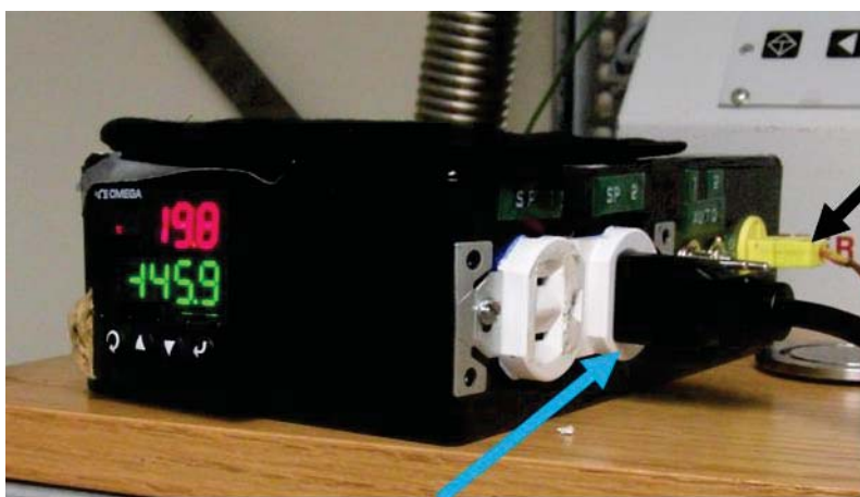
FIG. A.29. PID temperature controller box. The blue arrow indicates the power cord from the \text{LN}_2 valve controller. The black arrow indicates where the ESD cryogenic reservoir TC cable plugs into the PID control box. The red value on the PID control box is the temperature ( ^{\circ}\text{C} ) read from the TC cable plugged into it. The green value is the target temperature ( ^{\circ}\text{C} ). For more information on the PID box, read its separate documentation.
