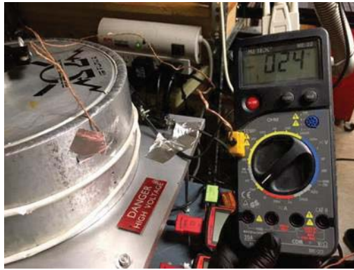
FIG. A.32. External temperature measurements—Aluminum tape is used to attach the TC to the chamber and is read with the multimeter.
