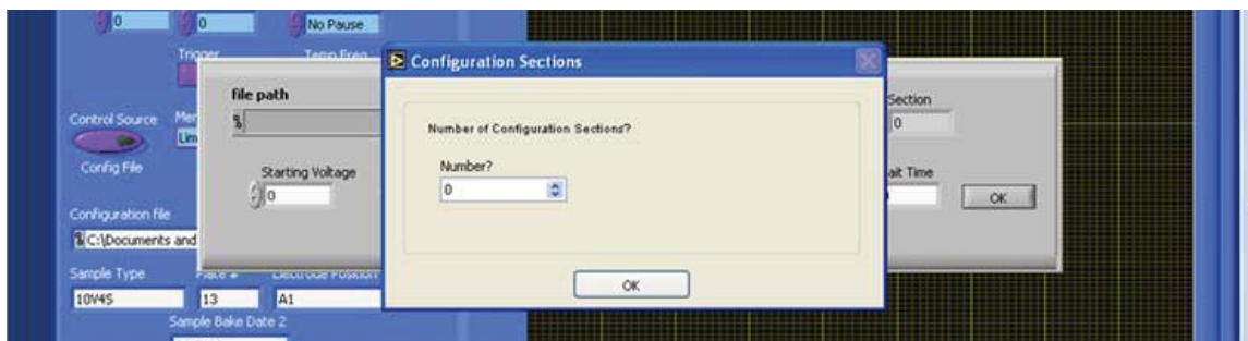
FIG. C.6. Configuration Sections window. 0 is entered if a previous configuration file is going to be used. Enter 1 if a new configuration file is to be created. Select 2 if there needs to be two sections created in the configuration file, e.g. , a ramp up to a wait voltage for a time-dependent run.
