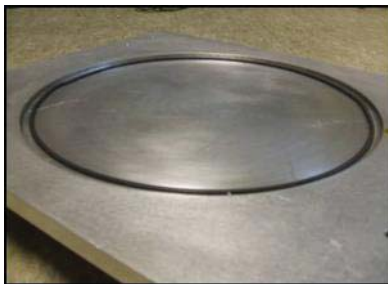
FIG. A.7. O-ring seated around recessed portion of base of chamber.
