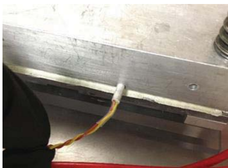
FIG. A.23. TC connections in the ESD chamber. Left- TC partially inserted into cryogenic reservoir. Right- TC electrodes circled in red on the ESD electrode plate.
