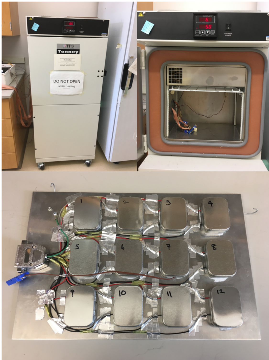
Figure 9. Thermal chamber (top two photographs) with one of three ceramic thermal electric plates (bottom photograph) for use in DTA. Plant tissue from individual black walnut trees would be placed in every cell, except cell seven (control), on a ceramic thermal electric plate and then placed in the thermal chamber for the analysis. Design developed by D. Gibeaut and T. Einhorn, (WSU) for DTA.
