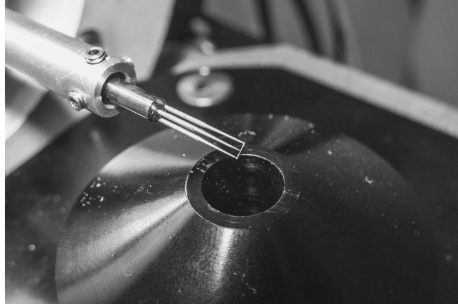
Fig. 3.1: TSI 1240-20 hot-film X-probe installed on the modified probe support on the calibrator
