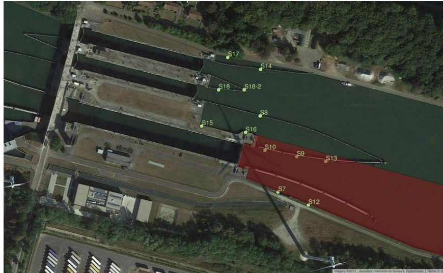
Figure 4. Aerial view with indicated in red the shadow zone of receiver S16. Source of background picture: Google Maps Satellite.
