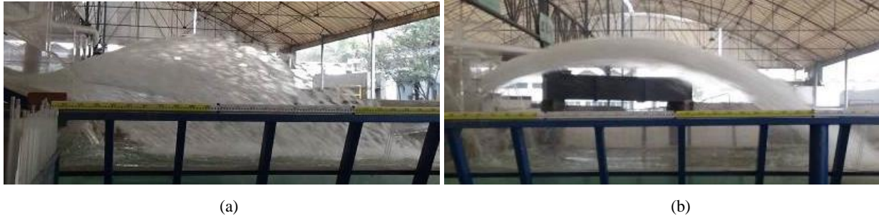
Figure 4. Comparison of typical jet diffusion between (a) leak-floor and (b) conventional flip bucket ( R = 30\text{m} ).
