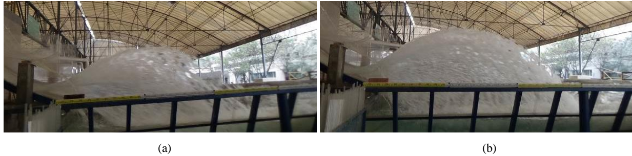
Figure 5. Effect of B_1/B_2 on jet flow pattern ( R = 30\text{m} , \theta_1 = 0^\circ ): (a) B_1/B_2 = 0.42 ; (b) B_1/B_2 = 0.54 .
