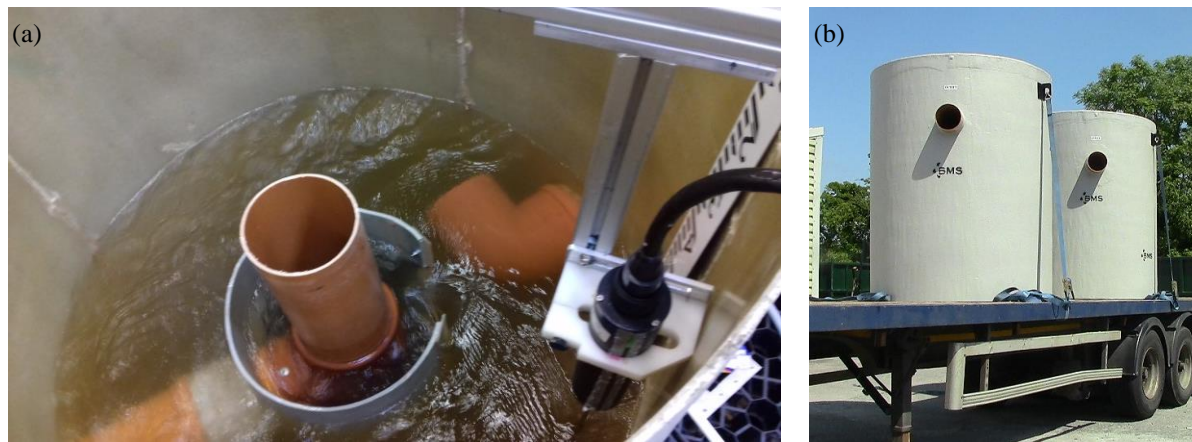
Figure 1: (a) Stormbreaker Defender chamber with Acoustic Doppler Velocimetry (ADV) probe used in this study and (b) Stormbreaker Defender (Model C) (image courtesy of Butler Manufacturing Services http://www.butlerms.com/ ).
