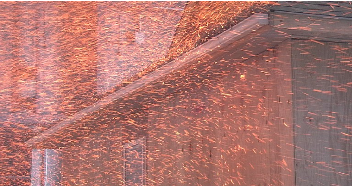
Figure 2. Ember storm produced in the IBHS research facility. Photo: Jack Cohen, USDA Forest Service and IBHS.
