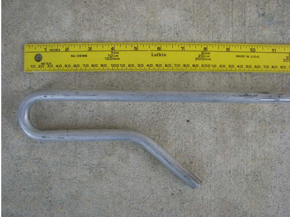
Figure 1. Distal end of telescopic, aluminum swan pole (3.2-cm crook gap) made of marine- grade aluminum rod (0.6-cm) used to capture flightless mute swans in the lower Potomac River and upper Chesapeake Bay, Maryland, USA, 2005–2008.
