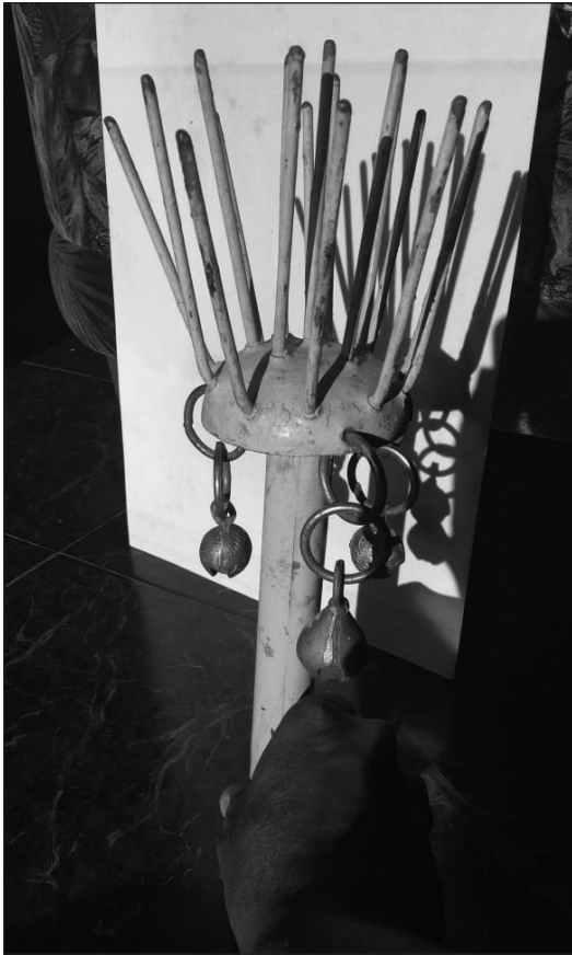
Figure 9. The Ghanti Kathi , a semi-circular surface having nails with blunt points and bells, and attached with a wooden stick 2–3 m long. The device, developed by our research team, produces sounds while walking and can also be used as a nonlethal defensive weapon against sloth bear ( Melursus ursinus ) attacks.
