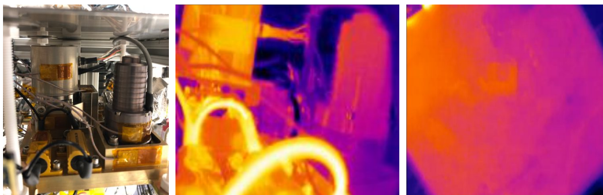
Figure 15. Flir Lepton IR images of the cryocooler, micro-pump, and HX plate. (Left) camera view. (Middle) IR camera view. (Right) Bottom of the HX plate
