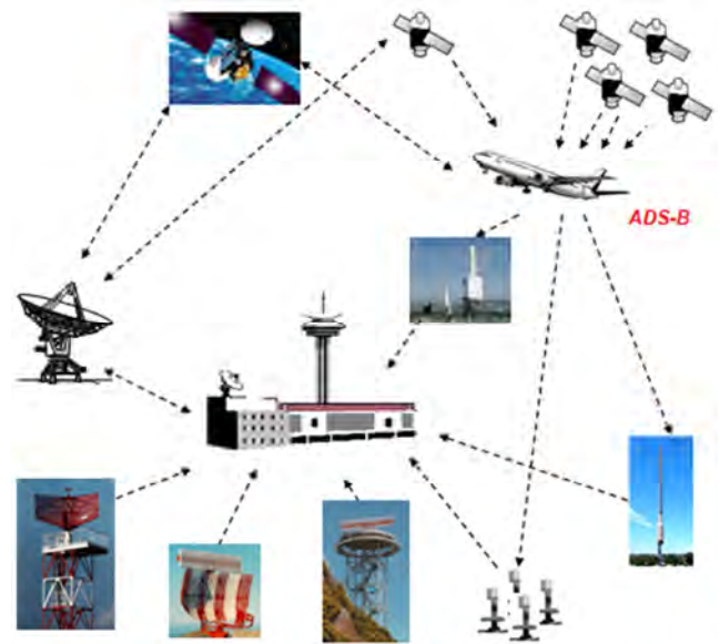
Figure 5. An Example of an Air Traffic Monitoring System.
