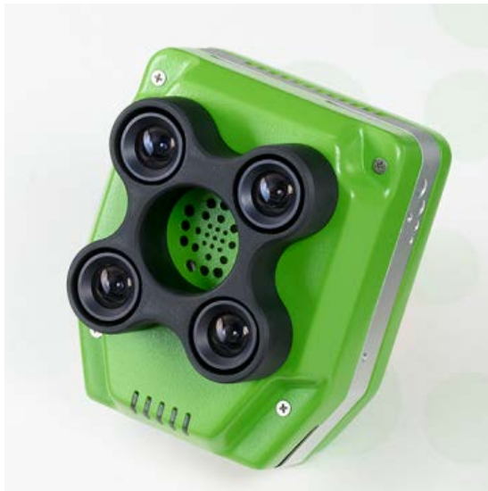
Figure 10: Chassis of stock Sentera Quad multispectral imager with custom band filters before modification by Sentera and NASA for use in space.
