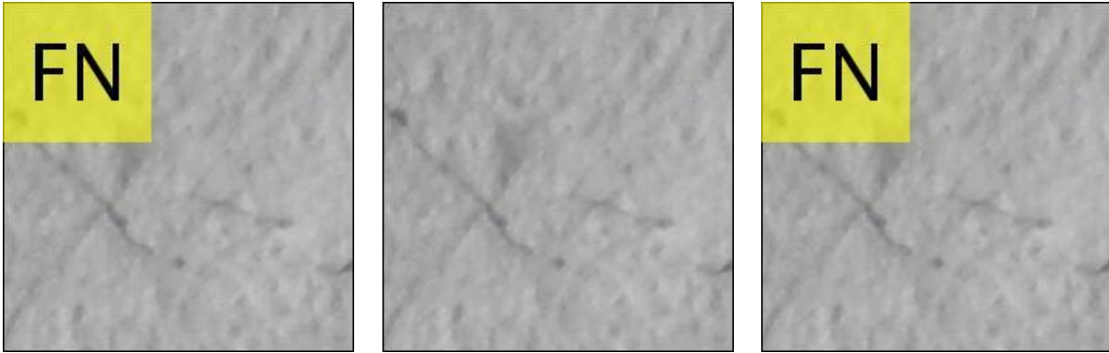
591 Figure 12. DCNN results for a crack of width 0.08 mm: (a) FT mode, (b) TL mode, and (c) CL mode
