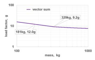
Figure 2: ESPA Mass Acceleration Curve
