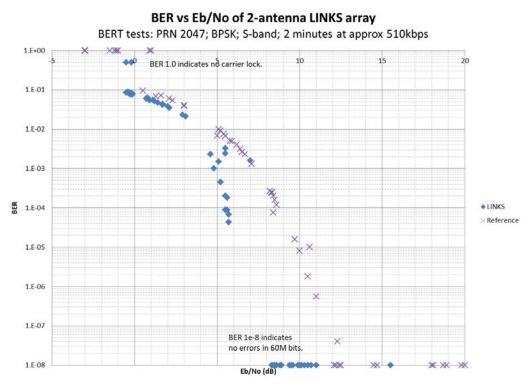
Figure 7 BER vs Eb/N0 chart of ATLAS LINKS for S-band Coded Downlink
