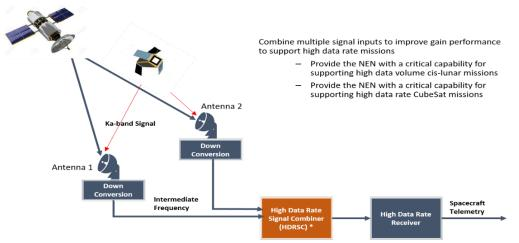
\*High Data Rate Signal Combiner (HDRSC) technology to be developed (orange box)
