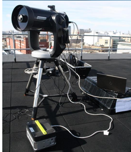
Figures 1a (top) and 1b (bottom). NODE Engineering Model and the Portable Telescope for Lasercom, respectively. Image Credit: Derek Barnes and Cadence Payne
