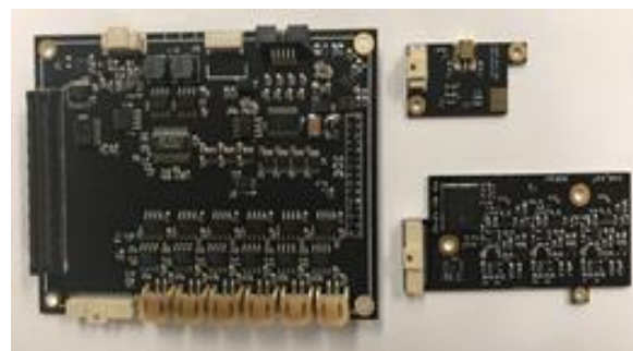
Figure 11: Daughter board, 90mm x 70mm (left), TOSA board (top right), and PD board (bottom right)
