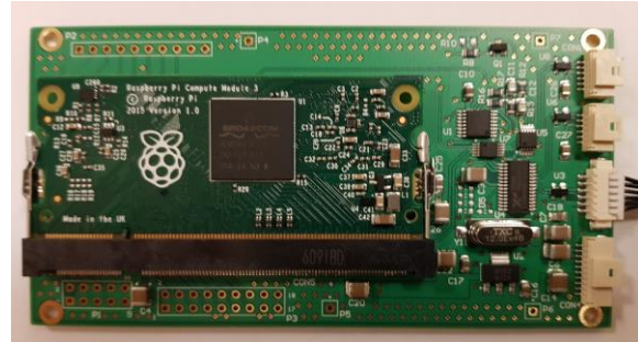
Figure 9: CPU Board (105mm x 55mm)
