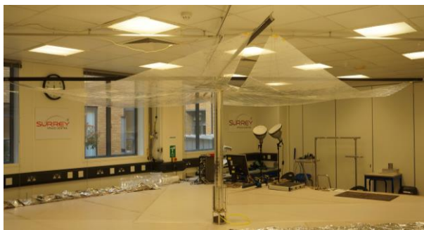
Figure 10. InflateSail Inflatable Mast and Drag Sail Deployment Test
