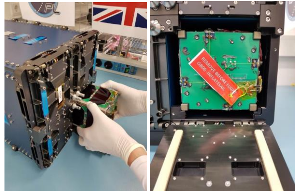
Figure 15. InflateSail Being Integrated into the ISIS QuadPack
