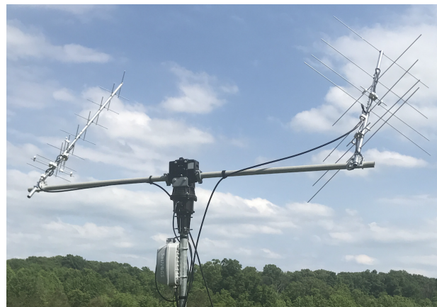
Figure 13: Corey Shields KB9JHU ground station #2 with commercial rotator with UHF and VHF antennas.
