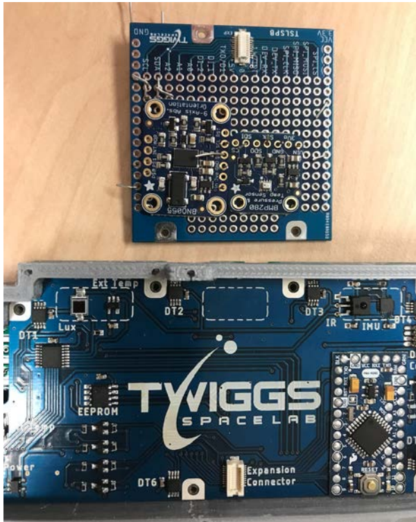
Figure 4: Twigg's Space Lab Primary Board (Bottom) and Secondary Board (Top) Separated
