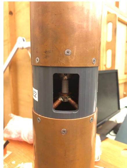
Figure 14 Broadband Dipole Viewing the RF Feed Built at Cal Poly.
