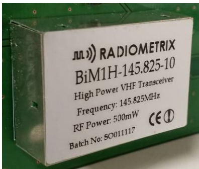
Figure 2: VHF transceiver payload of BIRDS-2 project
