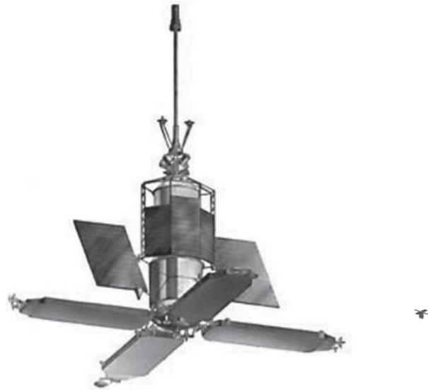
Figure 6: Tselina-2 satellite from 1980's (payload mass 1120 kg) versus 6U CubeSat (payload mass 6 kg).
