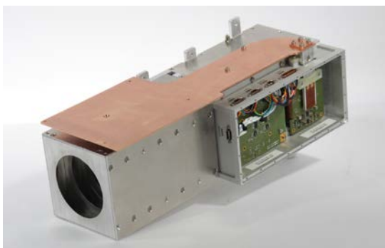
Figure 6. Engineering model of the O 2 A-Band limb sounder including a straylight baffle
