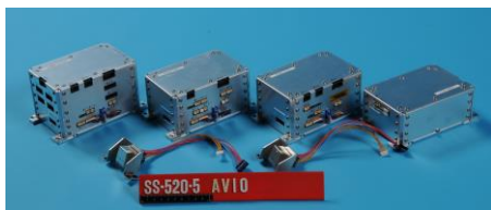
Figure 8: SS-520-5 COTS Avionics
