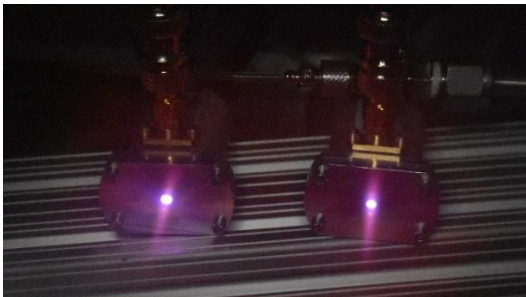
Figure 8: Pocket Rocket thrusters operating side by side in a vacuum chamber test.
