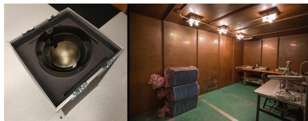
Figure 6: Shield can (left) and copper room (right) used for resolution test
