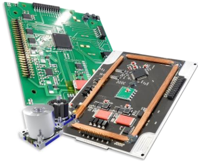
Figure 5: QUBE actuators and ADCS PCB showing an uncovered reaction wheel and a magnetorquer, which is placed on the back of a solar panel
