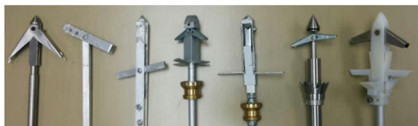
Figure 9. Harpoon projectile prototypes and evolution.
