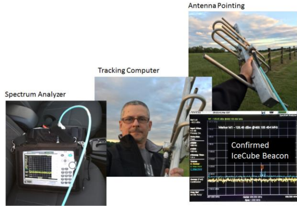
Figure 20: Crude "Ground System" Used to Detect IceCube Signals after Loss of Communications
