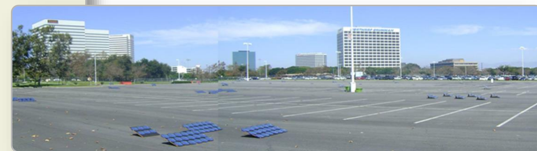
SPARC mirror targets deployed at the Raytheon parking lot in El Segundo, California.
