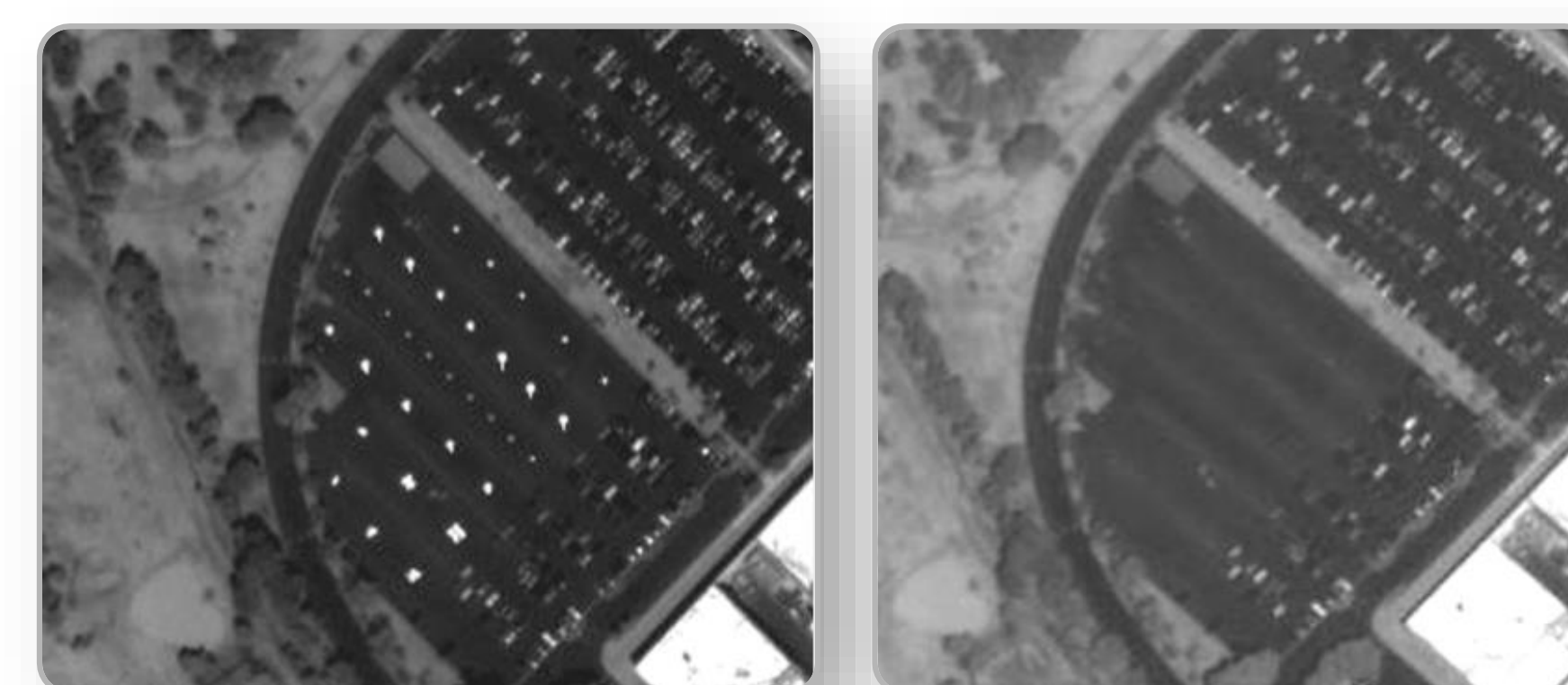
The IKONOS images show two consecutive collects inside and outside the mirror's field-of-regard, illustrating the effectiveness of isolating the direct solar signal. The sensor's response to each "solar star" provides a known effective at-sensor radiance for deriving radiometric gain coefficients.
