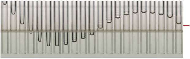
FIG. 1. A water meniscus falling and rebounding in a partially submerged glass tube with inner diameter of 6 mm. The immersion depth is 23 mm and the initial fill height above the free surface was 97 mm. The red arrow indicates the location of the equilibrium capillary rise for this configuration. See also video 1 of the supplementary material accompanying this figure.
