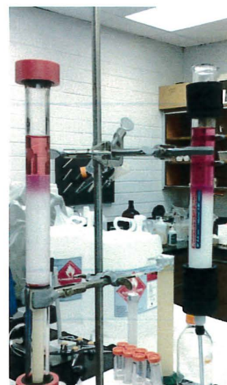
Figure 6: Columns used for column chromatography. Columns contain Capto Q or Capto700 resin.
