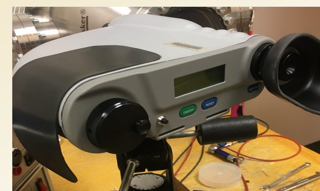
Optical pyrometer, used to determine temperature of silicone surface
