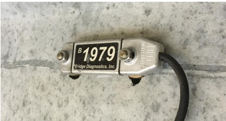
Figure 16. Strain Transducer Attached to the Bridge (Pickett 2017).
