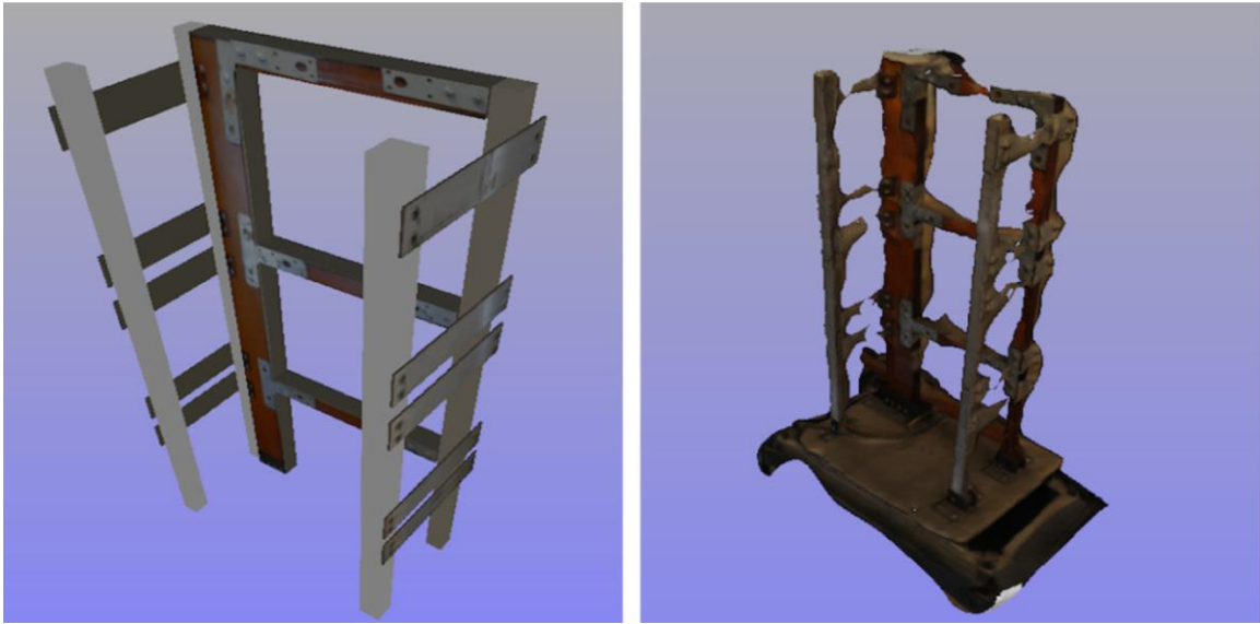
Figure 6. 3D models of the aluminum/acrylic structure using IM (left) and DSfM (right) modeling (Lattanzi and Miller 2015).
