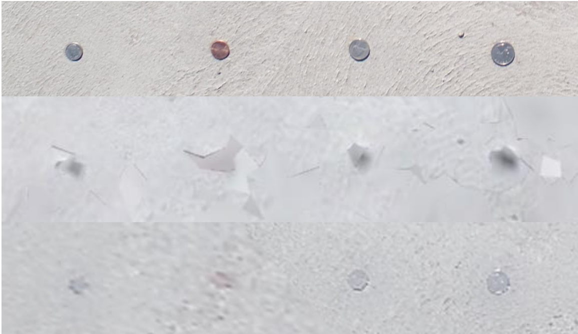
Figure 94. Drone photograph of coins placed on the Elwood Bridge (top); coins from the DroneDeploy model (center) and Agisoft PhotoScan model (bottom).
