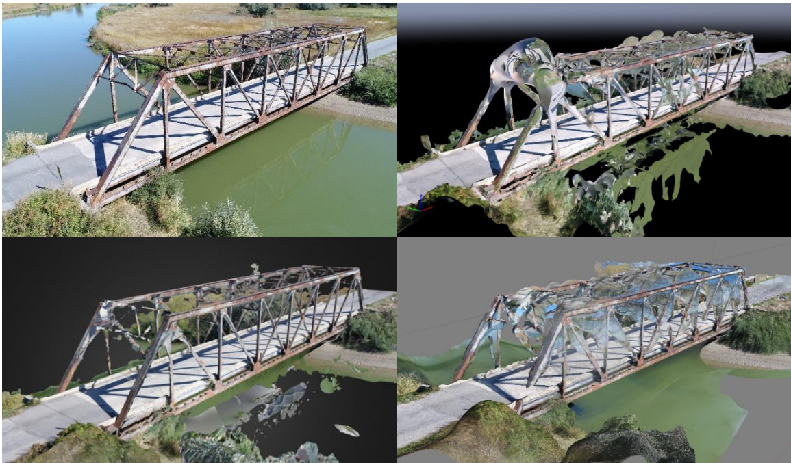
Figure 81. Photograph of the Trenton Bridge (top left) compared against screenshots of the Pix4D (top right), DroneDeploy (bottom left), and Agisoft PhotoScan (bottom right) models.
