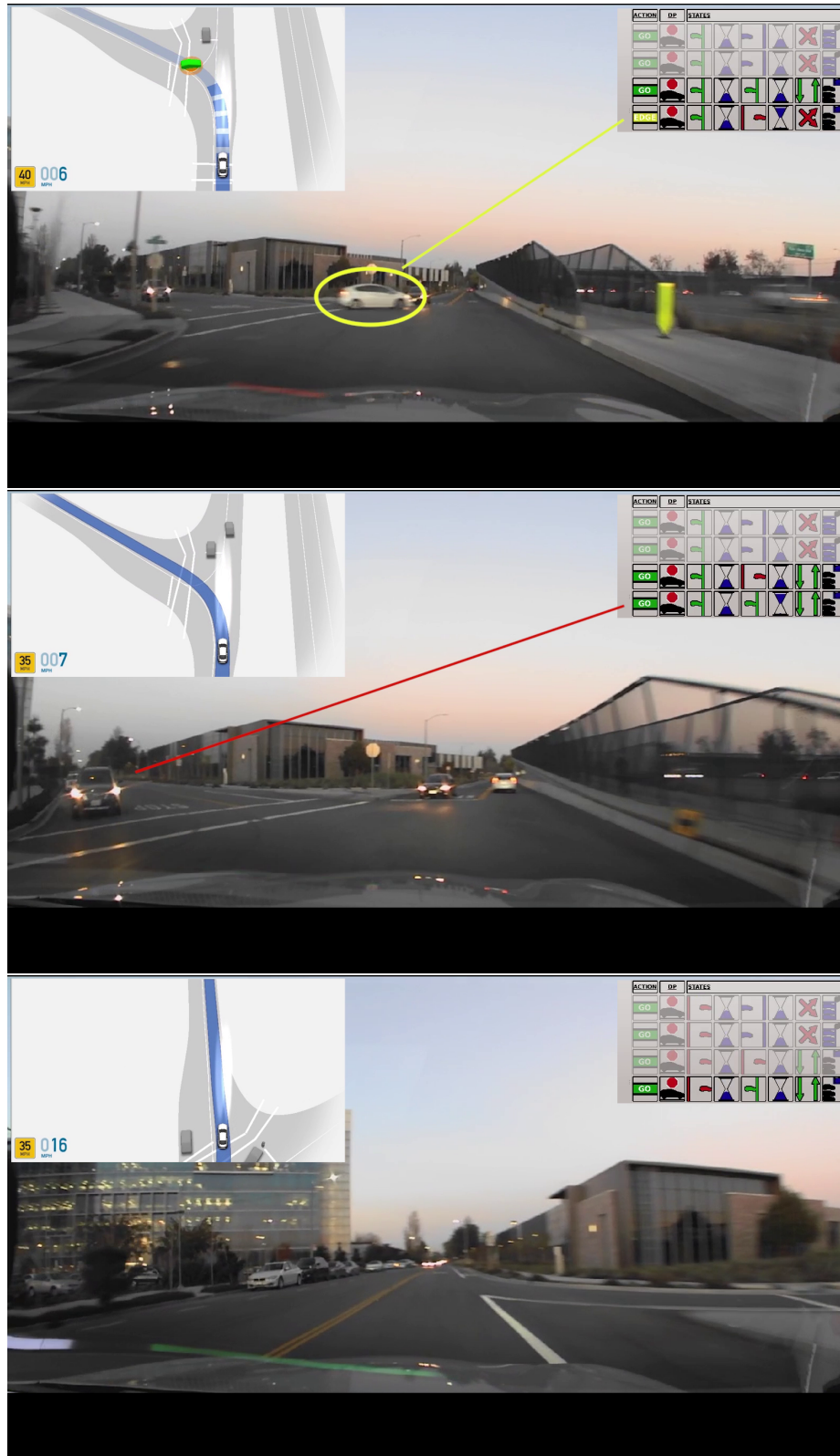
Figure 7.5: Experiment 3-Way Stop (Part 2 of 2) in Sunnyvale, California during 2017. This is MODIA, as part of a policy network, interacting with real traffic on a public road. The left corner shows a visual of the high-level route plan. The right corner shows a visual of the mid-level MODIA decision-making; each row represents one DC. Images provided courtesy of Nissan Research Center - Silicon Valley.
