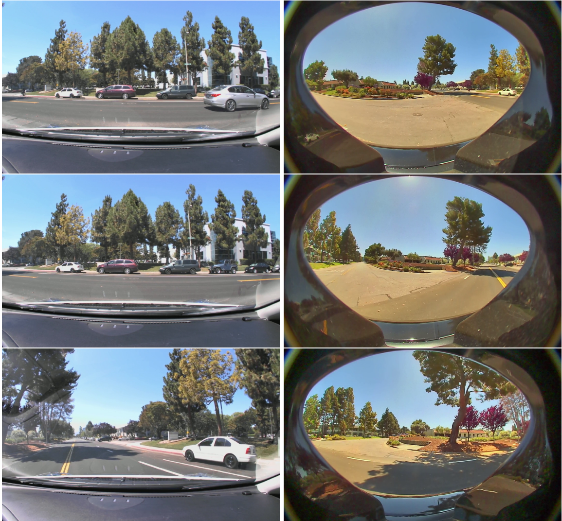
Figure 7.8: Experiment Partially Observable T-Intersection (Part 2 of 2) in Sunnyvale, California during 2017. This is MODIA, as part of a policy network, acting on real public roads with one staged researcher (partially observable left vehicle). The left column shows the front view and the right column shows the side view. Images provided courtesy of Nissan Research Center - Silicon Valley.
