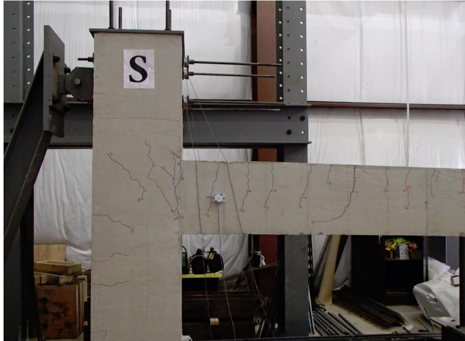
Figure 5.22: Cracks near the south column (Specimen 2)
