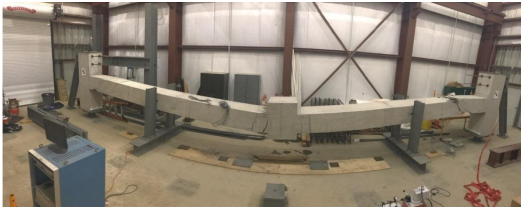
Figure 5.6: Specimen 1 condition at the end of testing after removal of force
