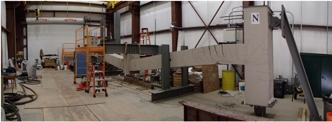
Figure 5.24: Specimen 2 condition at the end of testing after removal of force
