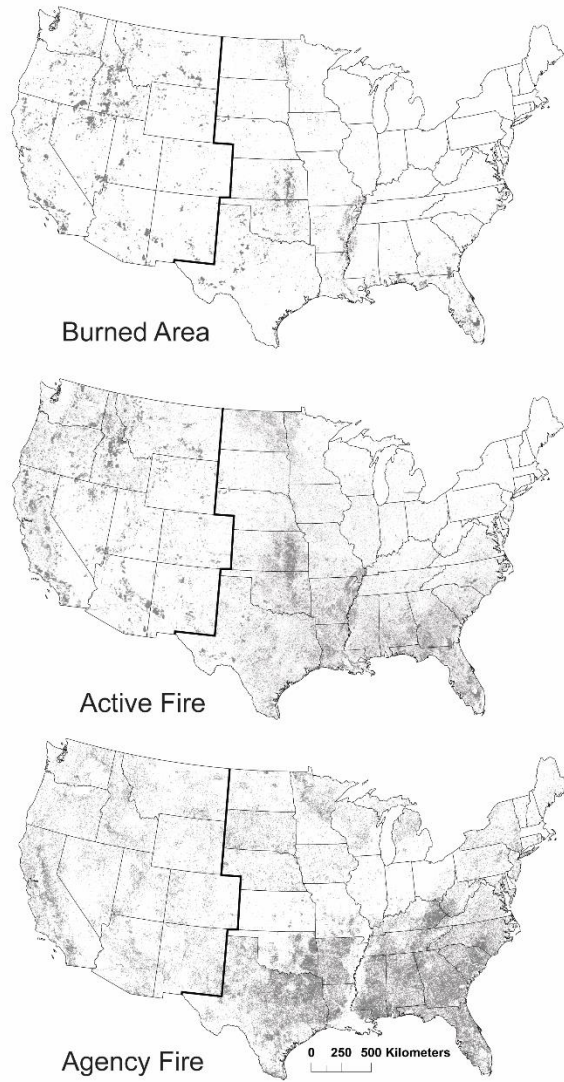
Figure 1.1: There are clear spatial disparities between A) the MODIS burned area product, B) the MODIS active fire product, and C) the agency fire records >1 ha. Agency fire product points and MODIS burned and active fire product pixels from 2003 to 2013 are shown in gray and a black line separates the eastern and western U.S. states. All agency fire point locations are the same size regardless of final fire size. Maps are in an Albers equal area conic projection.
