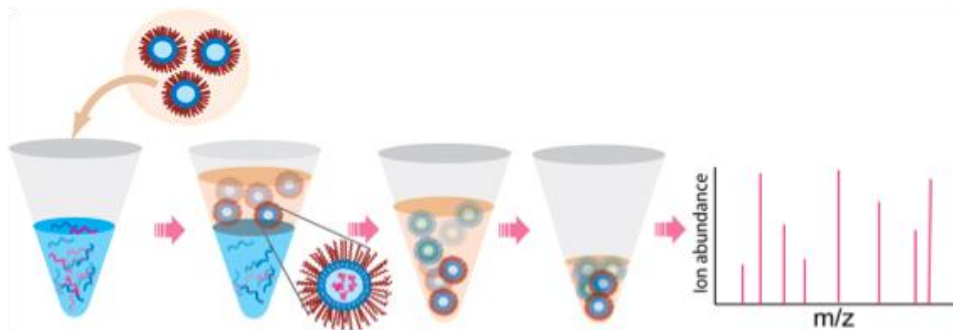
Scheme 1.9 Selective detection of biomarker peptide from a mixture using reverse micelle combined with MALDI-MS technique.
