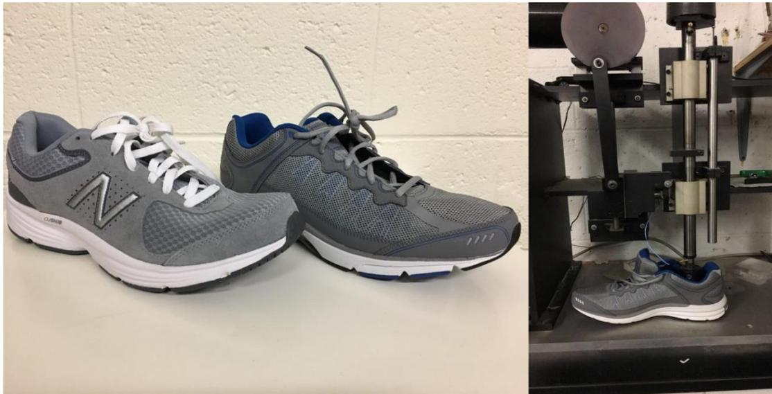
Figure 3.1: (Left) Neutral control (New Balance MW411v2) and variable stiffness shoe (Abeo Smart 3300) conditions used for this study. (Right) Impact testing of VSS. Shoe was positioned under the impact tester while a projectile with a mass of 8.5 kg was dropped from a height of 30mm. Load cell within the projectile measured projectile acceleration, force, and displacement.
